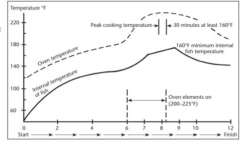
Figure 1. Typical internal fish temperature during a smoking cycle.
